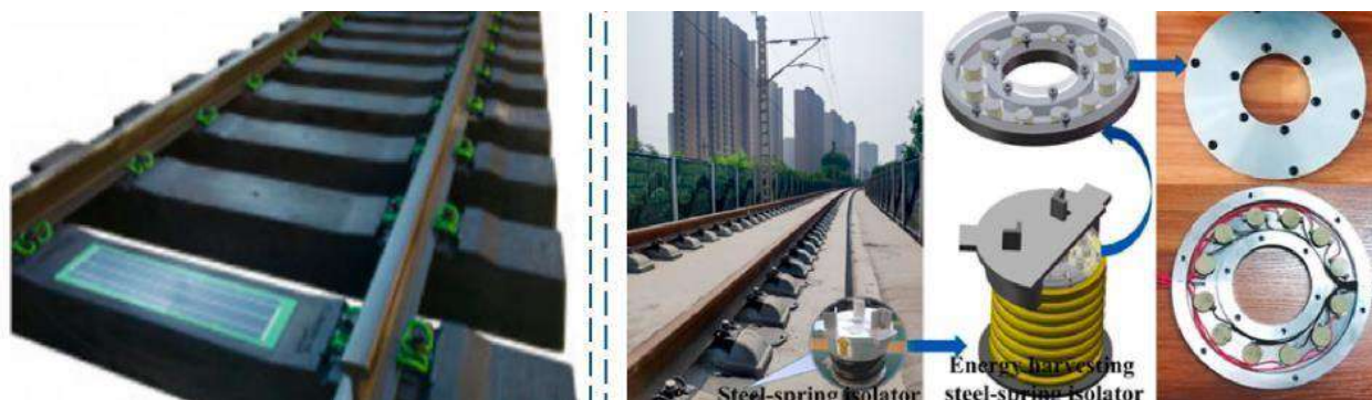
Fig.2.5. Green railways and PZT Stacks on Railway Tracks.
